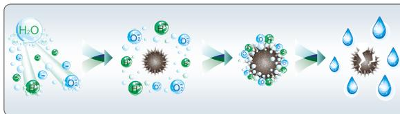
**Air Ionizer (Cold Plasma Generator):** this is able to reduce pollutants, decomposing their molecules using electrical charges, causing the water molecules in the air to split into positive and negative ions. These ions neutralise the molecules in the gaseous pollutants, obtaining products normally present in clean air. The device is able to eliminate 90% of the bacteria. The result is clean, ionized air, free of foul odours.
