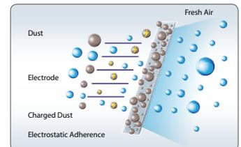
Operating principals of the **Electrostatic dust filter** (electrically powered).
